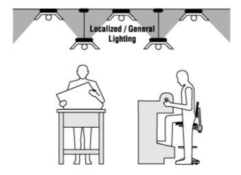
Local (or task) lighting increases light levels over the work and immediate surroundings. Local lighting often allows the user to adjust and control lighting and provides flexibility for each user.
