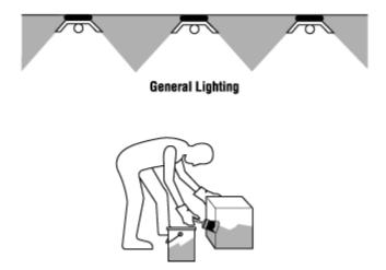
Localized-general lighting uses overhead fixtures in addition to ceiling fixtures to increase lighting levels for particular tasks.
