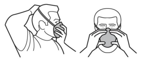
Figure 2: How to put on a disposable respirator
